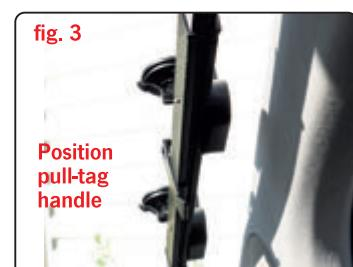
Remove the pull-tag from the transparent suction cup and retract it to the passenger side. Then installation is completed.
